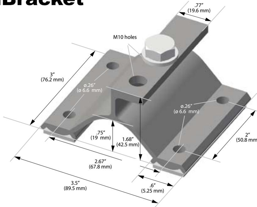
Part comes with M10 bolt and washer. Contact your distributor for information on other hole configurations.
